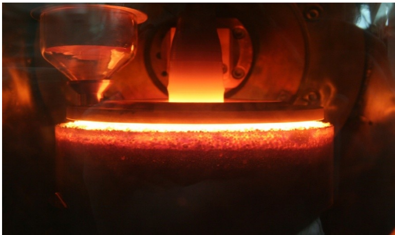
During the growth, the melt is embedded in unmelted silicon
