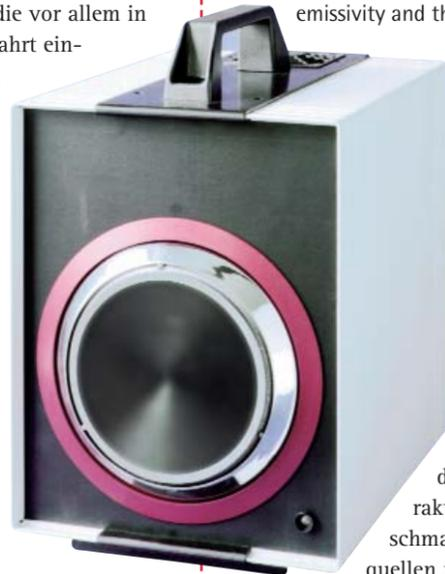
on the market. The temperature range of these IR emitters extends up to 250°C depending on the emitter type. All three calibration sources are wide-area emitters with an aperture of 100 millimetres. They are remarkable for their high emissivity and the particularly homogeneous distribution of the temperature over the radiant surface.
