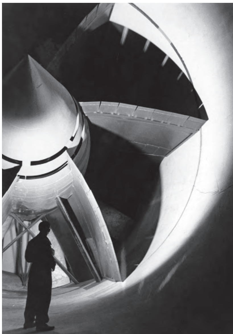
The driving unit of the "Great Wind Tunnel" spanning 8.5 m. The power generated by the engine reached 2,000 KWH
