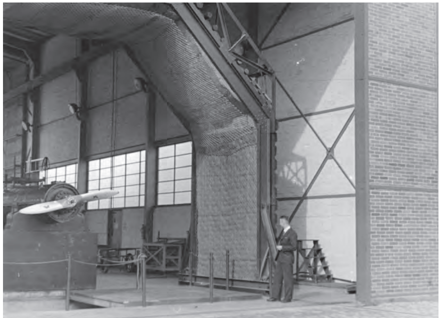
The tandem engine of a Dornier-boat sea-plane on the engine test bed
