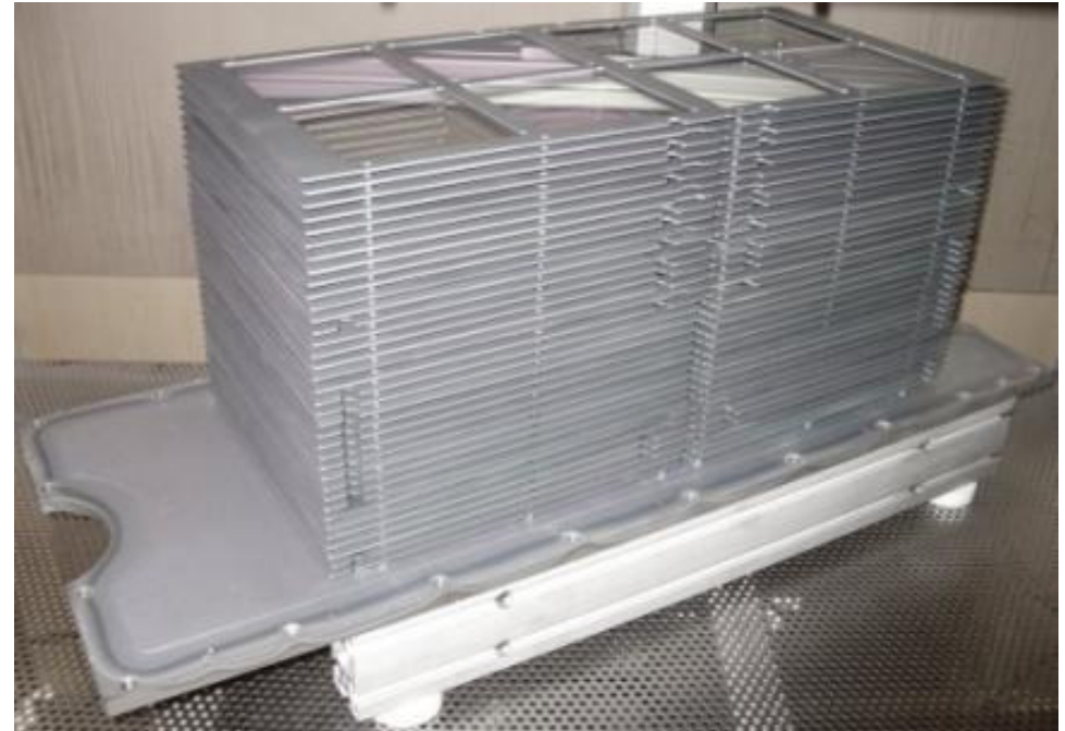
Beneq P400A reaction chamber with a stack of 100 x 100 mm 2 glass substrates.
